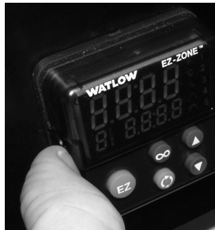
Pull out the tab on each side until you hear it click.
