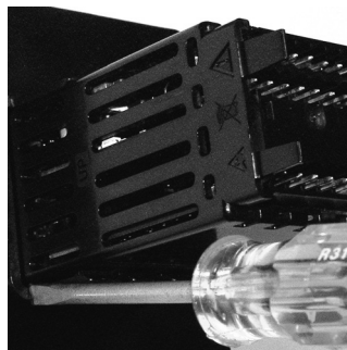
Place the blade of a screwdriver in any of the corner of the mounting collar assembly.
