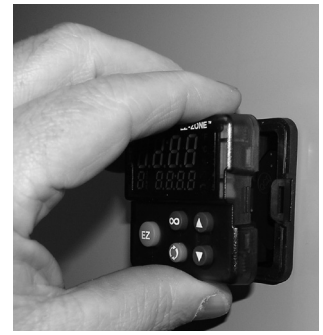
Grab the unit above and below the face and pull forward.
